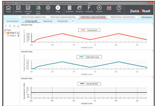
Step 1: Temperature control, stabilization Step 2: Determination of thermal strain
